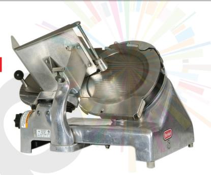
Always turn the power off and wait for the blade to stop spinning before placing and removing any meat, cheese, etc. from the carriage.
